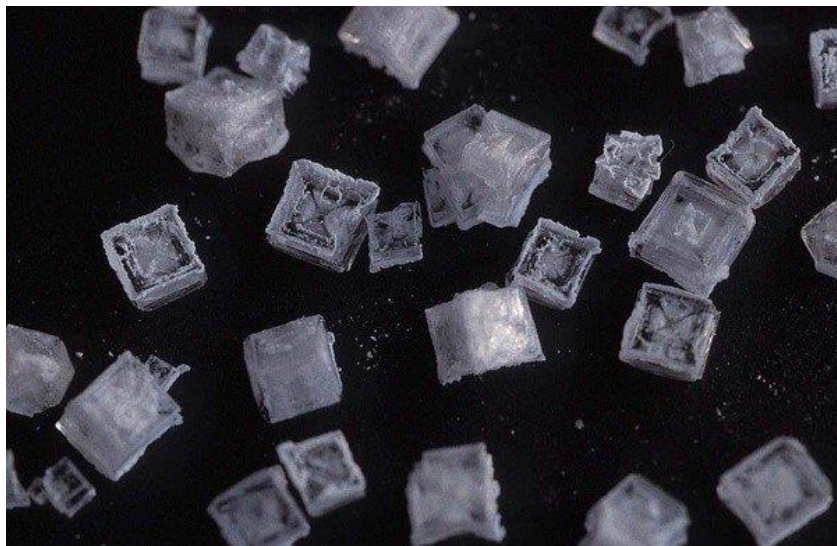
Figure 3: Crystal of Sodium chloride, also known as salt or halite, is an ionic compound with the chemical formula NaCl, representing a 1:1 ratio of sodium and chloride ions.
